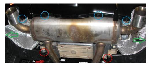
**2.5.** To install the rear mounts, simply remove the OEM 8mm bolt shown below.
