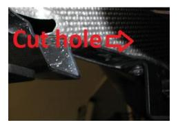
**2.9.** For the side mounts, we do something similar to the rear mounts. You can use either OE hardware or the M4 with a hole cut in the heat shield. These are installed later on (Section 2.14), but keep in mind for future reference.
