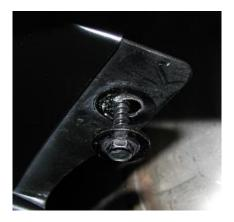
**2.6.** Grab one of the rear mounts and install it with the OEM bolt. Do your best to install the mount so it is pointing fore and aft (not crooked). Note orientation on car and slot positions.
