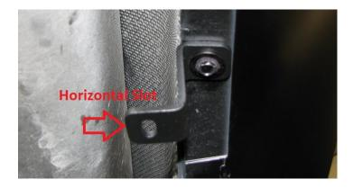
**2.7.** Alternatively, use the M4 supplied hardware through these points. This ensures the bolts do not vibrate loose over time. The below photo shows this hardware installed.
