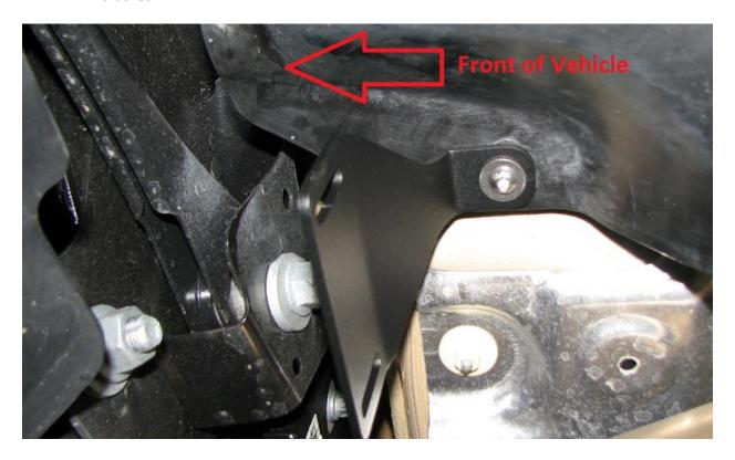
**2.14.** The final brackets to install are the side brackets. As mentioned previously, these can be installed with either the OE hardware, as shown below, or with the M4 supplied hardware. The bracket is installed below.
