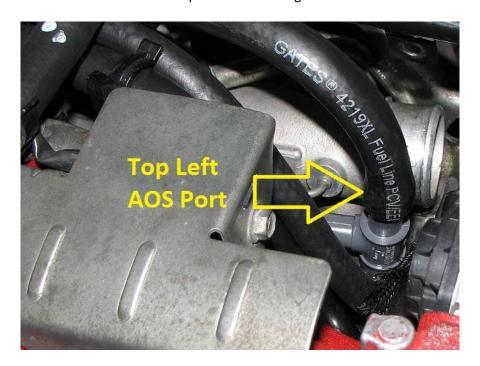
**4.10.** The below photo shows the top port on the tee (yellow) and the side port (orange) which is the drain, ran on car.
