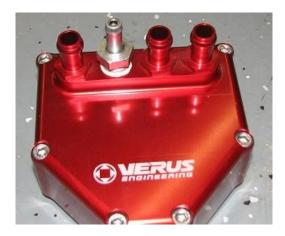
2.19. At this point, we can install the bracket onto the AOS and get it ready to install on car. Use the (5) M6x1.0 x 12mm Long BHCS and the (5) M6x12mm OD washers, and install the bracket as shown below. \*If you are installing the coolant kit, install the coolant plate as shown below.\* It is also suggested you install the coolant hoses now, skip to step 3 and read through these directions.
