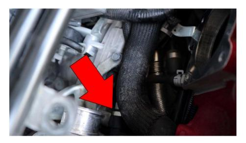
**2.13.** Below is a photo of the PCV T fitting with PCV valve on it which we removed in the above photo.
