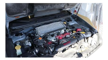
**2.3.** For this install, we have to remove the intercooler if you still have a TMIC (Top Mount Intercooler). Start by removing the (2) 12mm bolts that hold the vent tube on circled below in red.
