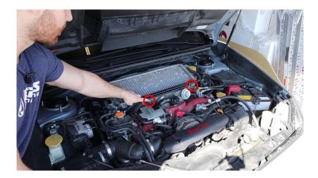
**2.4.** Remove the BPV by taking the two 12mm bolts off, shown circled below in yellow.
