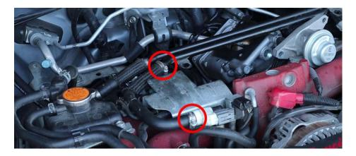
**2.31.** Cut an 18" section of 1/2" hose and install the hose as shown below on the PCV tube.
