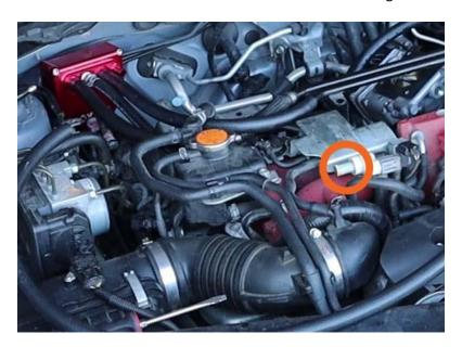
**2.34.** Install the other 9" section on the second intake port on the back side of the intake manifold as shown in 2.14 and circled in orange below.
