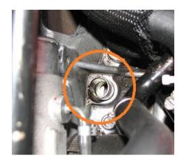
**2.17.** We now want to remove the PCV check valve from the piece shown in 2.13 by using a 19mm deep socket. This is also shown below.
