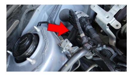
**2.23.** Install the factory bracket onto the AOS bracket by using the supplied M6 nut as shown below.
