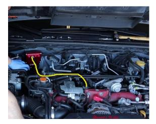
**2.27.** At this point, we decide to reinstall the wiring loom back onto the factory bracket as shown below. To do this, we need to slightly trim some of the electrical tape down by the firewall so that the wiring loom can reach the new mounting location. Be VERY cautious doing so as you do not want to cut into the wiring. **Note that the wiring loom needs to be flipped in order to reinstall it on the factory bracket.**
