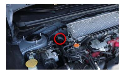
**2.22.** To remove the factory bracket (shown below), remove the 10mm bolt that connects to the bracket to the strut tower.
