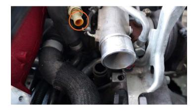
**2.35.** Now we need to tie these two sections together using the supplied 1/2" Y adapter.
