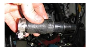
**2.29.** Taking roughly a 20" piece of 1/2" hose, we can install this hose on the 1/2" side of the adapter that we just installed. Route the hose in the best manner possible and install the other end onto the far left 1/2" barb on the AOS.
