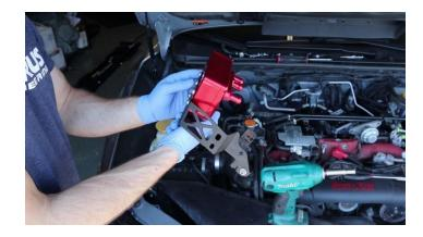
**2.24.** Using the supplied M8x1.25 bolt and washer and the M6x1.0 x 12mm BHCS and M6 x 18mm OD washer, install the AOS and bracket assembly as shown below.
