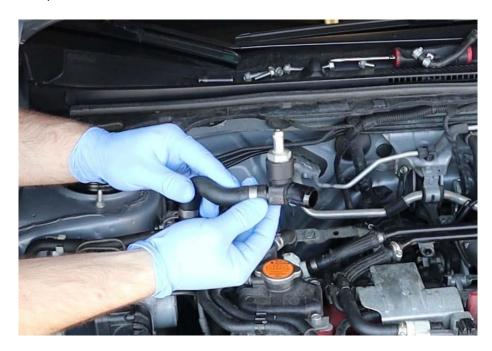
**2.14.** Below is a photo of where the PCV T fitting with PCV valve were removed. These locations are circled in red.
