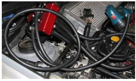
**3.5.** Install the shorter hose onto the overflow as shown below. Try to spill as little coolant as possible by using a clamp.
