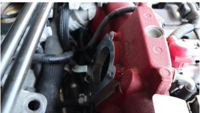
**2.10.** We can now remove the hose from the barb that is attached to the intake manifold. This is located directly below the throttle body, circled below in yellow.
