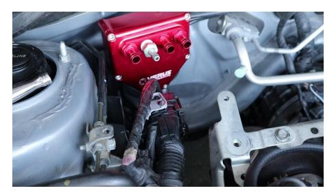
**2.28.** For the engine block location, we can reuse the factory hose or the supplied 3/4" hose with the 3/4" to 1/2" adapter as shown below. Install this in the location as shown in 2.15.
