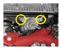
**2.5.** Undo the charge cooler silicone hose by loosening the clamps, circled in blue below.
