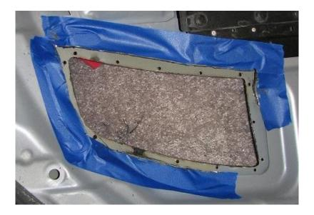
**2.22.** Using sanding discs/roll-locs, sand the edges of the skin and structural metal to avoid cuts and remove all sharp edges.
