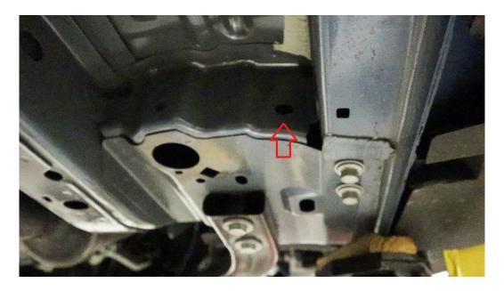
**2.6.** Using the instructions below, install the hex body rivet nut into the center of the slotted hole.
