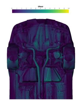
The rear diffuser is doing little for downforce production. This specific diffuser looks to be used to help with drag reduction by helping fill the wake region behind the car. The diffuser is also used to help with rear differential cooling with the ducting above the diffuser.
