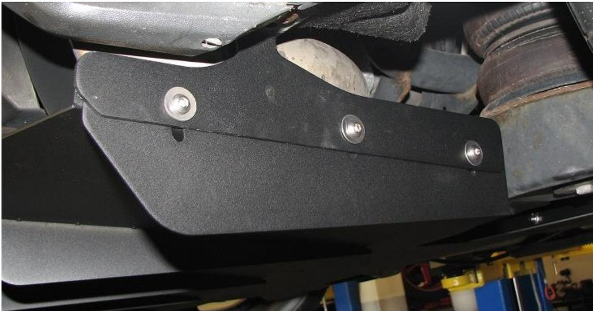
**2.18.** Once all bolts and nuts are installed, tighten all button head cap screws to approximately 10 ft-lbs. The serrated nuts, when tightened, will resist backing off.
