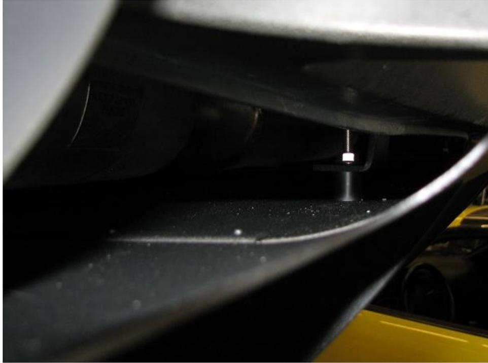
**2.17.** Moving to the mid-brackets, we install the bolts, washers, and nuts.
