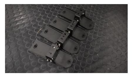
**3.17.** Once the brackets are assembled, it is now time to loosely install these on car. Do so by feeding the 20mm long SHCS and 18mm fender washers through the cutout in the bottom bracket and loosely installing them into the rivet nuts we installed earlier. Note that you want a little play both forward/rearward and side to side initially. Also note the "shorter" side is towards the front of the car.
