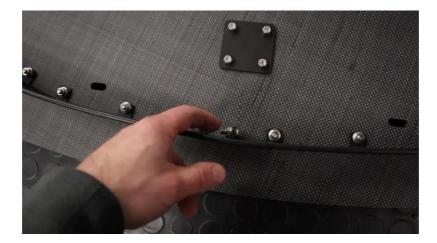
**4.4.** Loosely install the air dam onto the splitter using the 20mm long BHCS and 18mm fender washers on the bottom side and then a serrated nut on the top side. Only install the nuts hand tight initially. Once the splitter is on car, we can make final adjustments for the air dam before fully tightening it down. Below is what the splitter should look like before getting installed on car.
