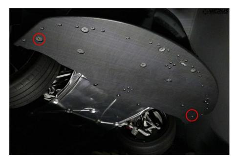
**5.8.** With the splitter fully installed, we can now make final adjustments for the air dam. Do so by pressing the air dam up against the front fascia, as shown below, and tightening the BHCS on the bottom side with an impact. The serrations on the nuts will grab the powdercoat and will tighten if done properly.
