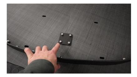
**4.3.** Once the splitter halves are attached, it is now time to loosely install the air dam. Start by attaching the air dam halves together by using the 12mm long BHCS, 12mm washers, and serrated nuts. You can make sure these two bolts are 100% tight at this point
