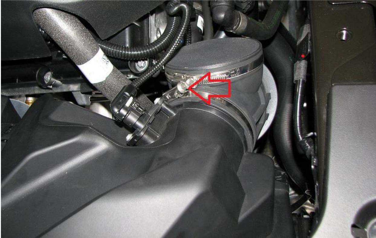
2.4. Remove the (4) intake filter box clamps, these are pointed out with the (4) yellow arrows.
