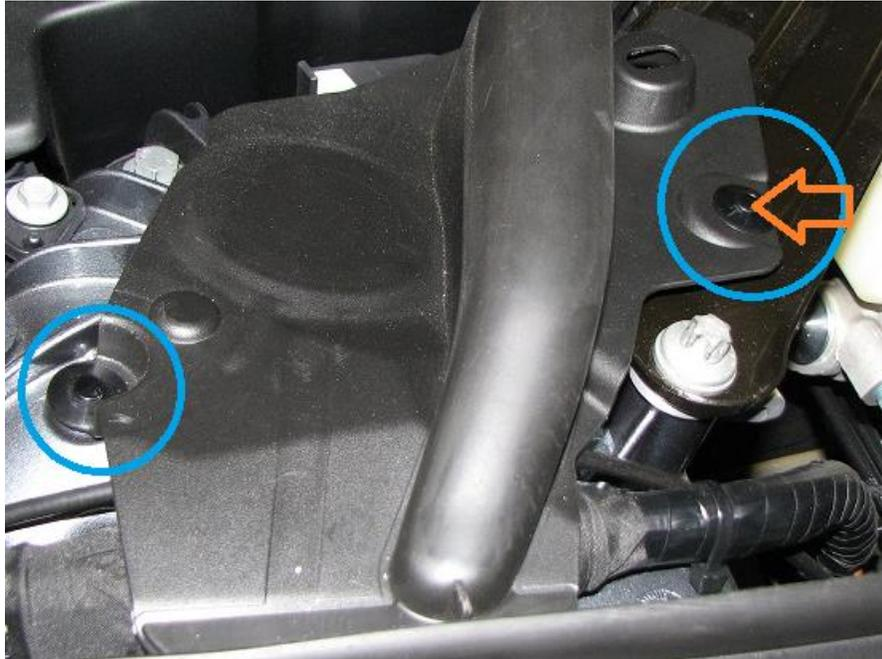
2.6. Once the rivets are removed, pull up on the cover as it presses into the center of the strut tower. You will have a similar picture below at this point.
