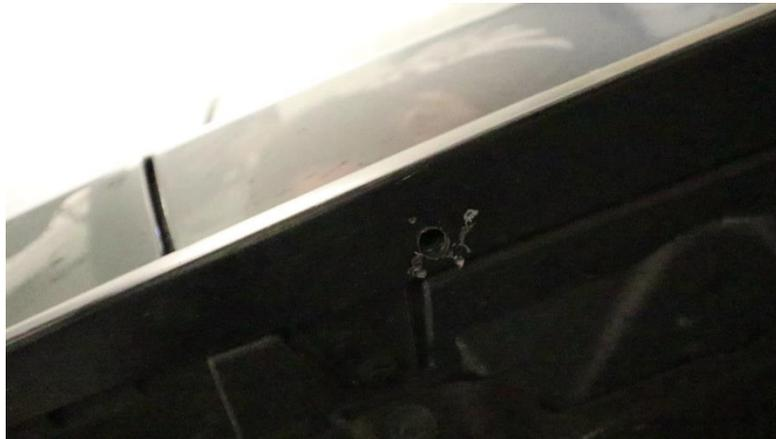
**2.6.** At this point, you need to decide if you want to install the side splitters with the plastic screws or the suggested method of installing rivet nuts into the factory side splitter. We chose to go with the rivet nut method.
