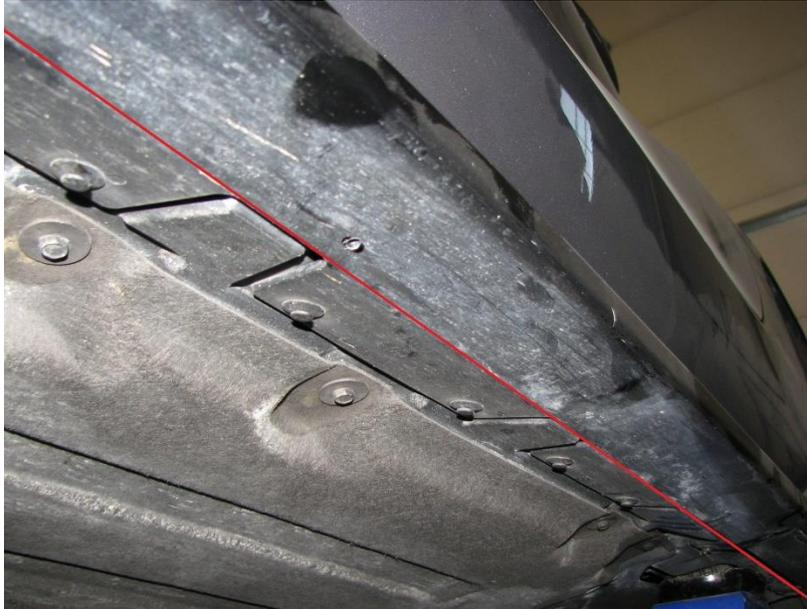
**2.4.** Once you have the side splitter positioned where you want it, using the side splitter as a template, grab a Sharpie or paint pen to mark the locations for drilling.
