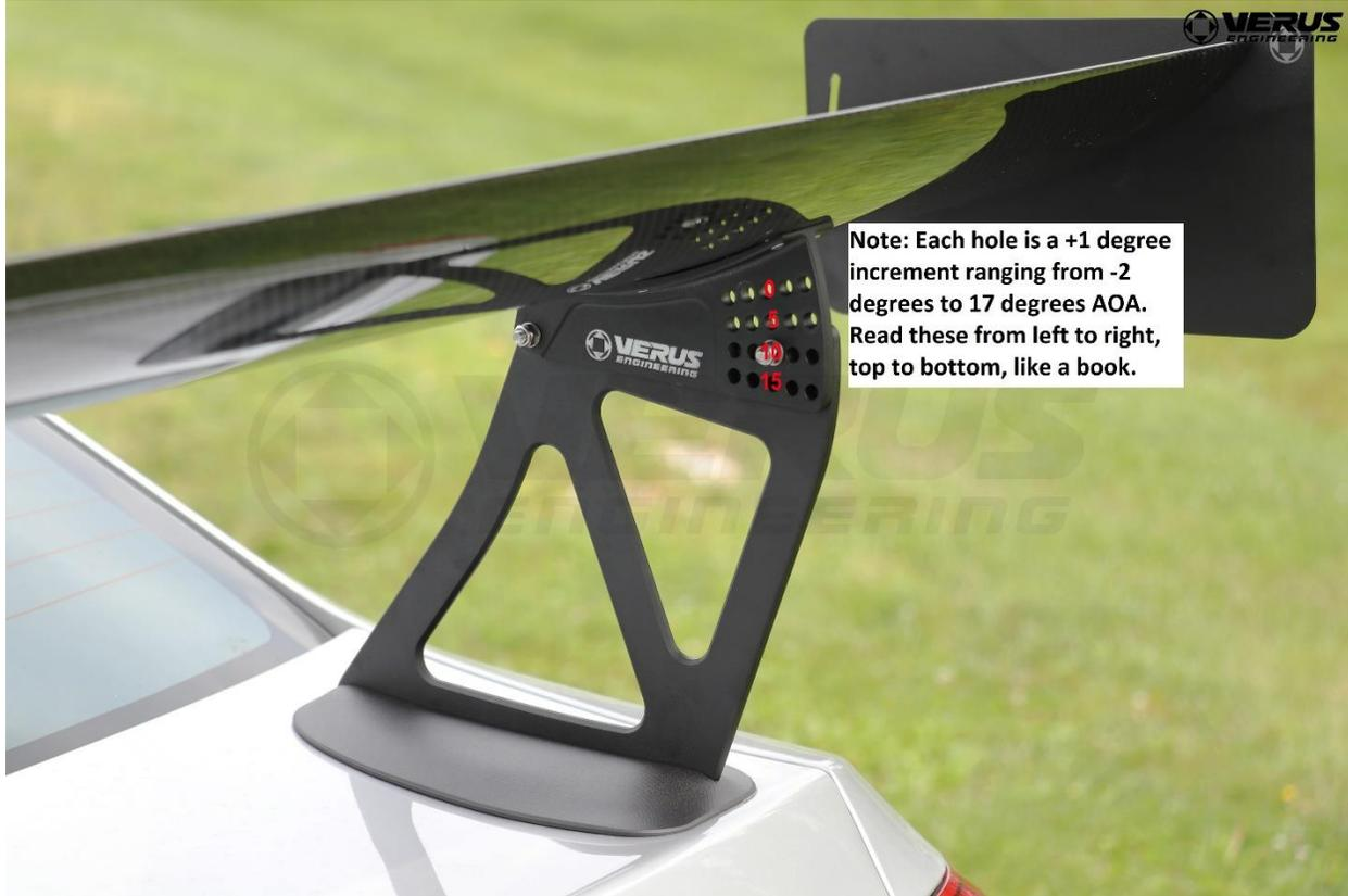
**2.14.** Lastly for the wing, we will install the end plates using a 2.5mm allen wrench and a bubble level. We recommend the endplates be installed parallel with the ground.
