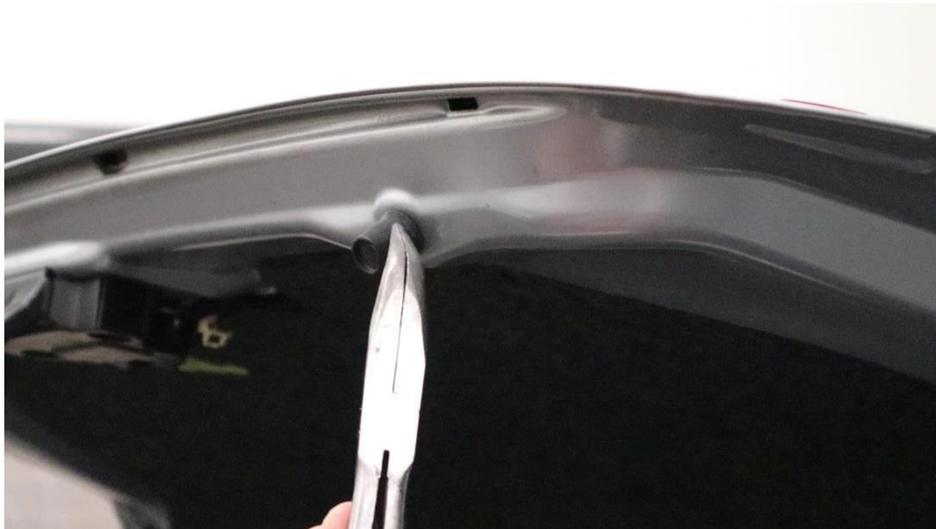
**2.15.2.** Once the bumper is removed, you will be left with a hole that you will step out to 3/8" with your step drill bit.
