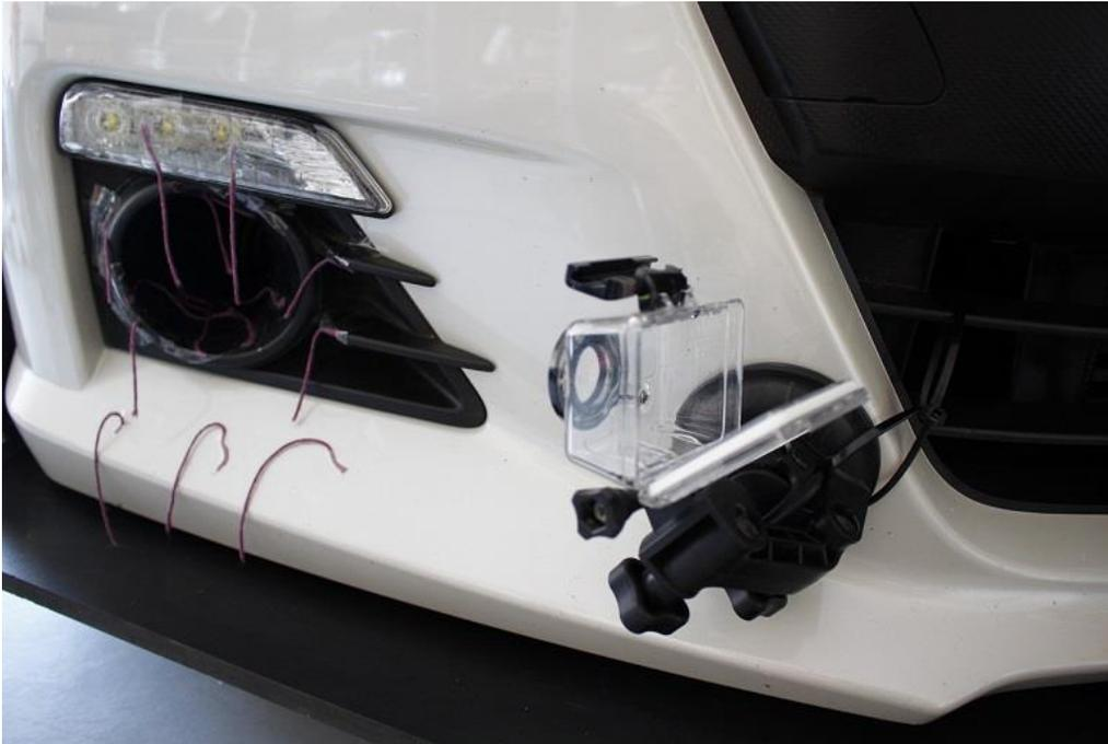
Figure 3.1: Test Setup for Tuft Testing
