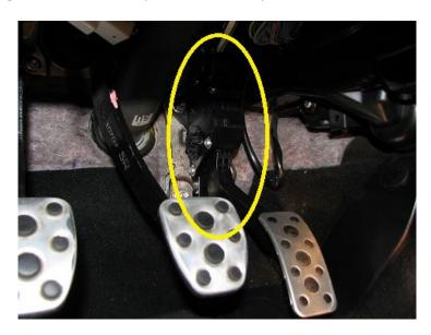
**2.5.** We will start with the throttle pedal assembly. Remove the two 12mm nuts, circled in red below.
