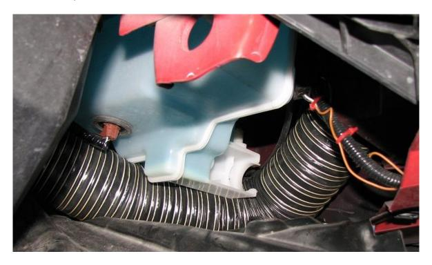
2.29. We will begin working on locating the fender liner duct, also referred to as the pancake duct by some. This duct will stick through the fender liner as shown below. This photo is taken from the front of the vehicle. Utilize a 3" hose clamp on the fender duct as well.
