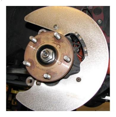
2.11. With the backing plate and the carbon duct installed, you may note that the speed sensor hits on the carbon duct slightly. Mark this location and remove the backing plate.
