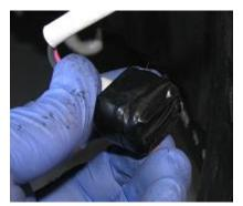
2.24. Place the fog light bracket around the duct and then the duct/bracket assembly into the hole where the fog light used to reside. Using the OEM screws, tighten the bracket down. The plastic fog light should have a little play but not a lot.
