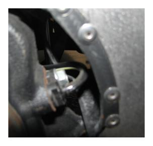
2.12. Using your mark as a guideline and one of the two strips of foam, wrap the wire to protect it against damage.
