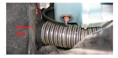
2.30. These hoses can be cut shorter for a more direct route if the washer fluid reservoir is removed, we supply the longest hose necessary for an OE install. Shown below is a more direct routing of hose after cutting took place.
