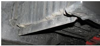
2.21. The fender liner is removed with various styles of plastic rivets and push pins, using your best judgement and the plastic removal tool, remove these.
