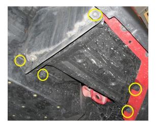
2.22. With fog lights installed, we need to remove the two Philips head screws circled in yellow below and unplug the connector from the fog light.
