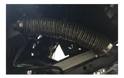
2.31. The below photo shows how we can snake the pancake duct through the fender liner; in between the engine bay and the fender liner. We recommend trimming the fender liner to allow use of the plastic push rivet but it is not necessary.
