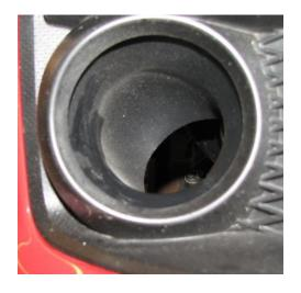
2.26. We can install the 3" brake duct hose now, use a 3" hose clamp on the fog light duct side.
