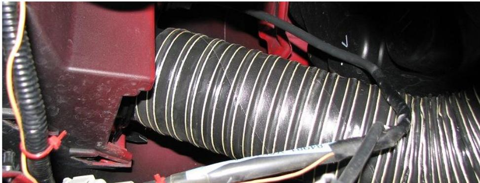
2.27. The hose is routed underneath the intake on the WRX. See below for a good picture of this.
