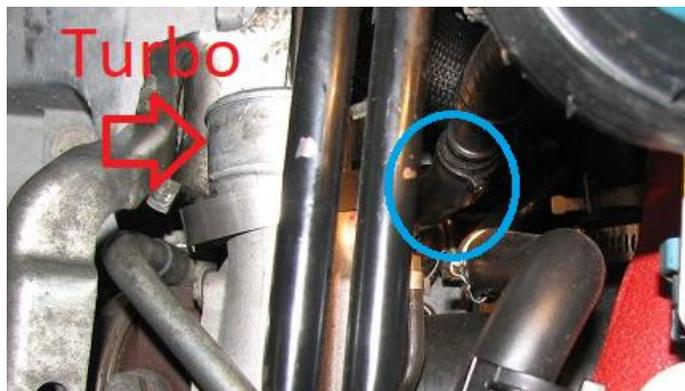
**2.10.** Below is a photo of the PCV T fitting with PCV valve on it which we remove above.
