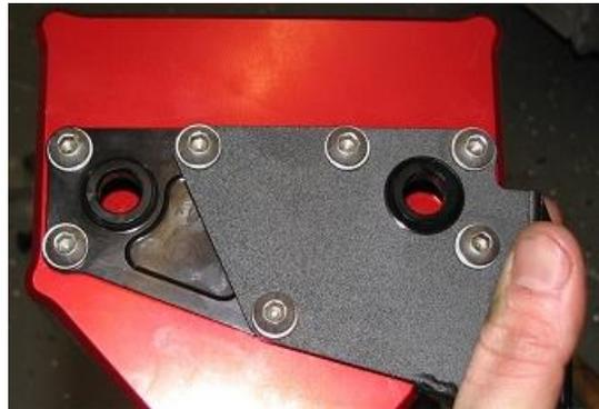
**3.2.** We recommend installing the banjo bolts and banjos before the unit goes onto the car. It is a good idea to install the hoses with clamps as well as it is difficult to reach once the AOS is installed on car.
