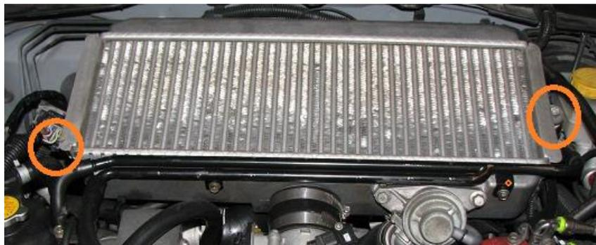
2.7. Remove the charge cooler from the car.
