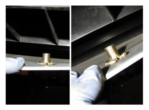
**2.17.** We have to install the smaller rivet nut in the front most hole due to the body being directly above it. To do this, we need to pull down the stock side skirt slightly. Remove the plastic rivet circled in red with a screwdriver and flat head.
