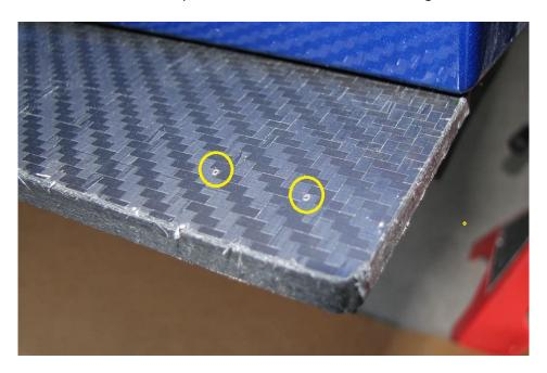
**3.2.** Using these holes, drill as straight through the side splitter as possible with the 3/16" drill bit.
