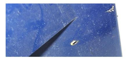
**2.9.** Using a stepper drill bit or a 1/4" then 3/8" drill bit, open these holes to a final size of 3/8".
