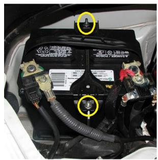
**2.4.** Fully remove the battery from the engine bay. With the battery out of the way, you will see a black plastic tray. Remove this as well which is shown in the below photo.
