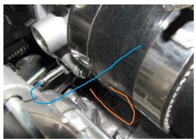
**4.5.** We recommend using the two below ports for inlet/outlet of the AOS coolant loop. Inlet and outlet do not matter to the AOS, so whatever looks and fits best is good.
