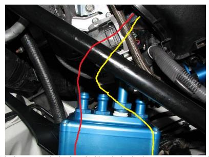
**4.9.** Install the hoses onto the banjos, clocking the banjos however seems best. Use the hose clamps (not shown) on each of the banjos to ensure the hoses do not leak.
