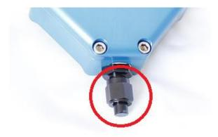
**3.2.** Remove the plug in the rear cam cover block off plate. This should be a 1/4" Allen wrench. This can be removed on car easily as well.
