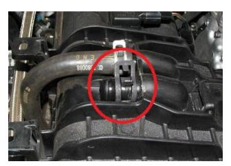
2.13.1.2. On the AOS itself, you will want to install the other 3/8" NPT to 1/2" hose barb adapter. Again, it is recommended to use Teflon tape, liquid Teflon, or a type of sealant to ensure leak free sealing.
