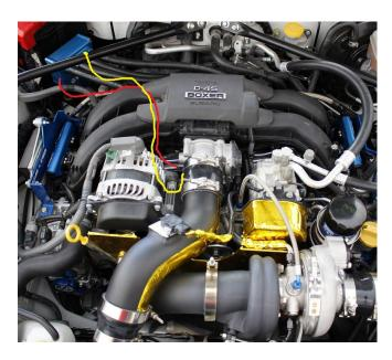
**4.8.** In the below photo, you can see how the hoses are routed under most of the connectors and harnesses.
