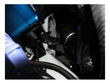
**3.6.** The optional automatic drain back system has been installed and is now functional. The AOS will automatically drain the oil back into the engine now, and will operate service free for multiple years.
