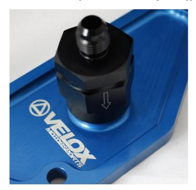
**3.5.** Using the supplied hose, install the straight hose end on the AOS, and the 90-degree hose end as shown below. Tighten these to 14 ft-lbs. *It is best to have the AOS loose on the bracket to allow some vertical play.*
