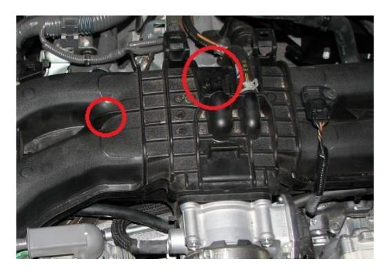
**2.7.** Remove the PCV valve using the 19mm deep socket, extension, wobble socket, and ratchet.
