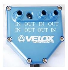
2.13.2.3. For routing, the below diagram depicts how to run the lines. The point from where the PCV valve used to go on the block, goes to the far left location (shown in RED below). The front block location is routed to the far right location (shown in GREEN below). The intake manifold hose goes from the inside left point to the intake manifold (shown in YELLOW below). The intake hose goes from the inner right point on the AOS to the intake tube (shown in ORANGE below).
