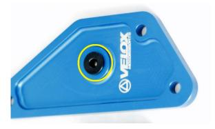
**3.3.** The check valve needs to be installed into this port we just removed. The arrow needs to point into the cam block off plate. Oil needs to flow into the engine, but we do not want the air to come out of the engine. **Install the supplied o-ring on the arrow side as shown below.**
