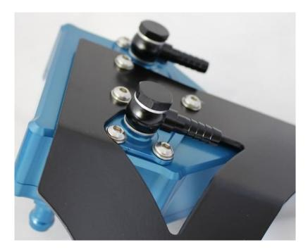
**4.4.** We will be using two of the three ports that are located near the throttle body for coolant inlet and outlet. Begin figuring out how you want to run the hoses as there are a few ways you can route the lines and how it can flow coolant through the unit. In stock configuration, you will have a short hose (shown in orange) that needs to be removed. The blue line is another coolant hose that should be disconnected from the throttle body as well.
