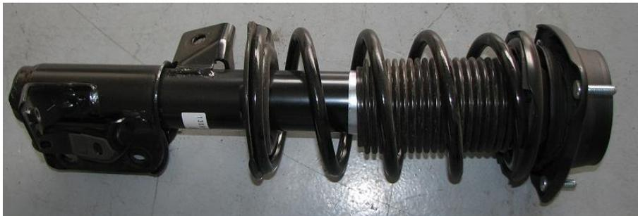
6.8. Using a spring compressor of your choice, compress the spring slightly so no pressure is on the top hat.
