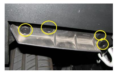
**6.7.** Grab the (4) thin washers on the top side of the fender liner once you remove the OEM wheel deflector. You will only need three of these pins and three of these washers for the install of the Verus Front Wheel Deflector.
