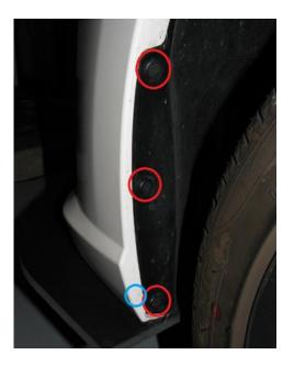
**6.5.** Once these four push pins are removed, you can pull the fender rearward. Looking from the top you will notice that each deflector push pin has a washer behind it on the top side. We will need these for re-install.
