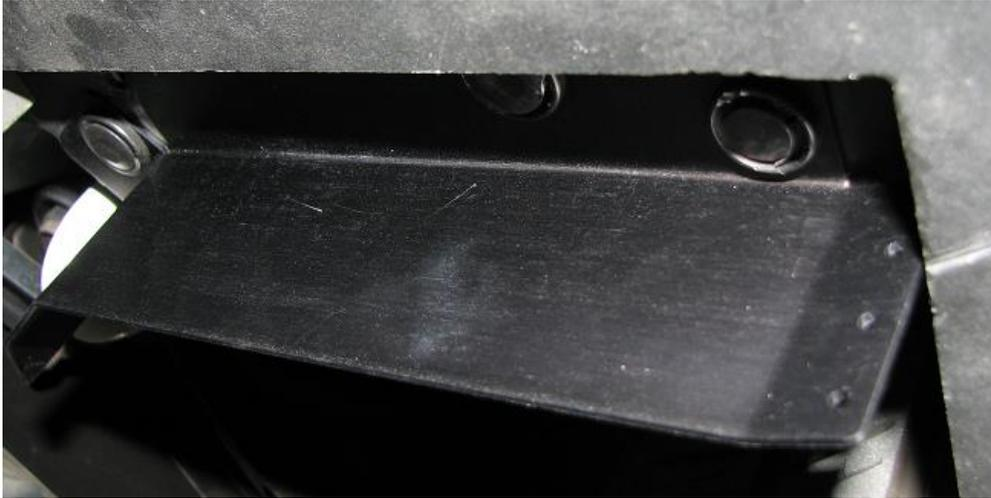
6.10. Next up is installing the add-on piece with the (3) bolts, (3) washers, and (3) nuts. The OEM add on is the smaller unit, while the Verus splitter add on is significantly longer unit. The install is fairly self-explanatory for each; however ever so slightly different. With the splitter add on, remove the closest M6x1.0 bolt and washer from the splitter with the 4mm allen wrench.
