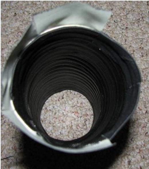
2.43. A fully finished duct is pictured below. The tape may not stick well to the hose due to the silicone/neoprene; however, once clamped it will hold well.
