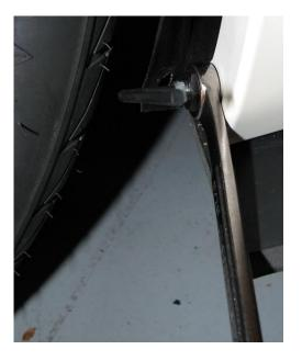
**6.6.** Using a flash light and the mirror, ensure that the rivet nut is fully installed. The Allen wrench will become harder to tighten as well. The rivet nut is fully installed when the flanges are flattened out as shown below. The threaded section should be near the install hole and tightening the Allen bolt will get significantly harder as well. If you do not fully install the rivet nut, the BHCS later on will have a hard time being installed.
