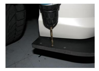
**6.10.** You have a decision to use flat head cap screws or button head cap screws on these bottom mounts. We went with the more stealthy flat head cap screws, but BHCS will work just fine. If using BHCS, skip this step, if using FHCS, use an 82 degree countersink, remove just enough material so the FHCS sits flush.
