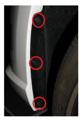
**6.4.** Once these push pins are removed, we will install the plastic rivet nuts. Using the supplied Allen wrench and the 9/16 wrench, we will assemble each rivet as shown below and then insert it into the bumper.
