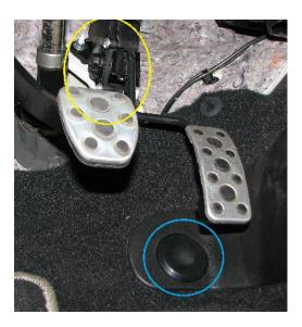
**2.5.** We'll start with the throttle pedal spacer. Remove the two 10mm nuts, circled in red below.
