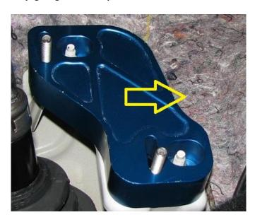
**2.11.** With the spacer torqued down, we can install the throttle pedal on the two bolts. You can adjust the throttle pedal vertically up and down. **We suggest starting with the pedal spacer tightened down in the middle of the slow.**
