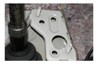
**2.8.** Before installing the pedal spacer, install the two hex head cap screws as shown below by inserting it through the opening location.
