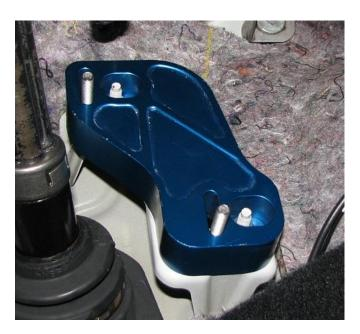
2.10. Tighten the OEM nuts to 6 ft-lbs. \*We recommend installing the spacer all the way to the right initially, giving the most space between the brake and the throttle initially.\*
