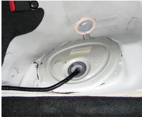
2.6. Use a screwdriver to pull up on the metal lid. With a razor, cut the black silicone to aid in removal.
