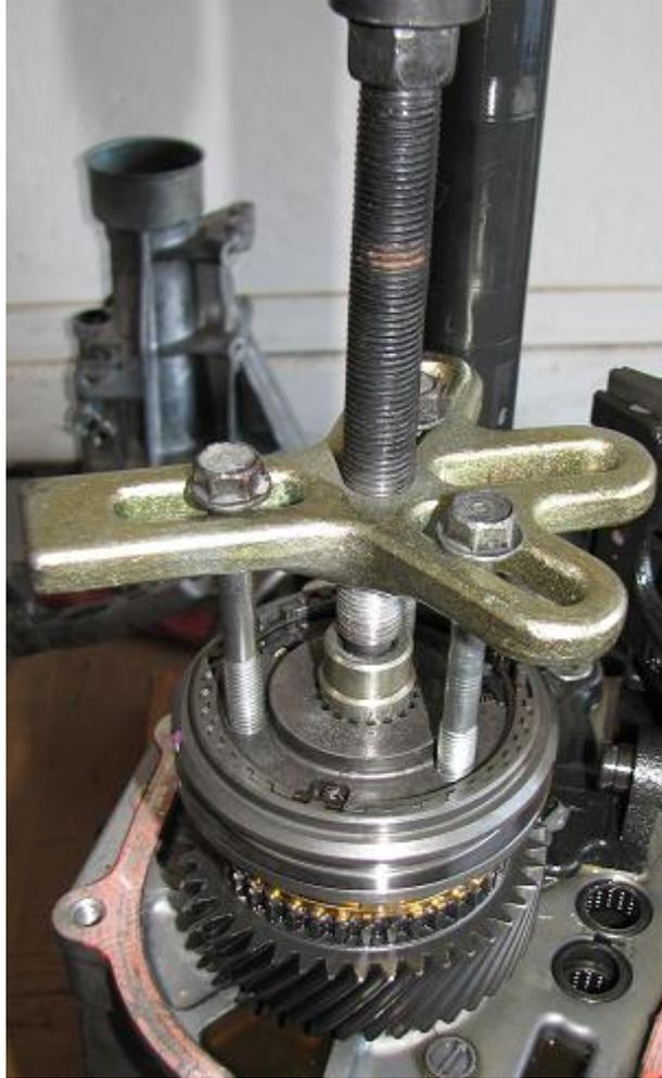
17) Remove 6<sup>th</sup> gear synchro and 6<sup>th</sup> gear after synchro hub has been pulled off. Remove the needle bearings that 6<sup>th</sup> gear rides on as well.
