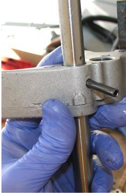
43) Place 6<sup>th</sup> gear, synchro, shift hub, and shift selector on the counter shaft and press the hub on. If you do not possess a press, you can hammer it on slowly but this is not recommended.
