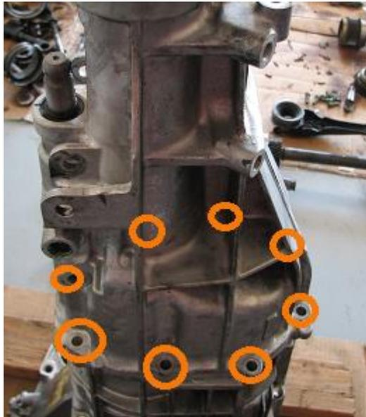
9) Using a hammer and/or a pry bar, tap up on the tail housing gently until the silicone holding it together breaks free.
