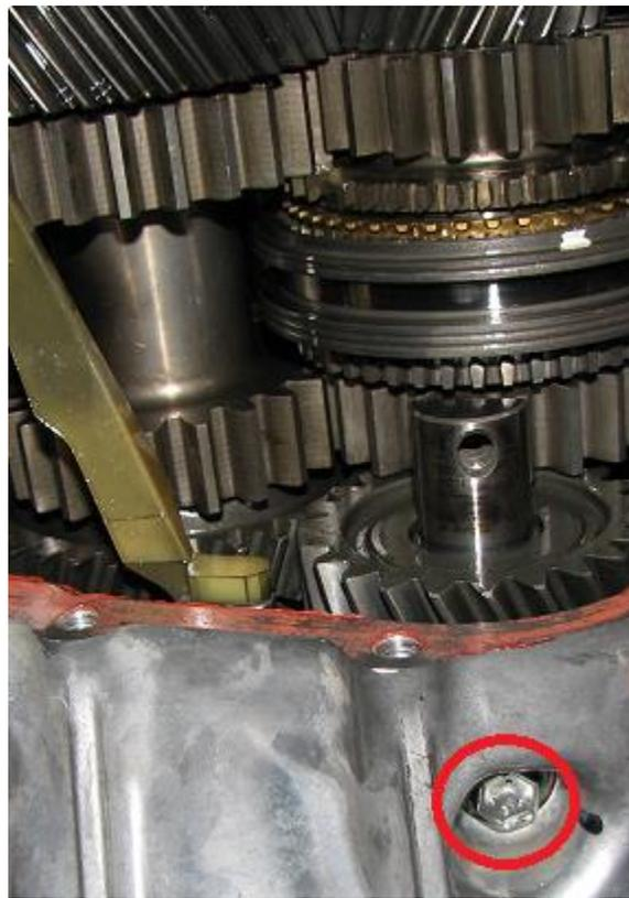
33) Flipping the transmission on its side and working from the engine side, install the two snap rings as shown below.
