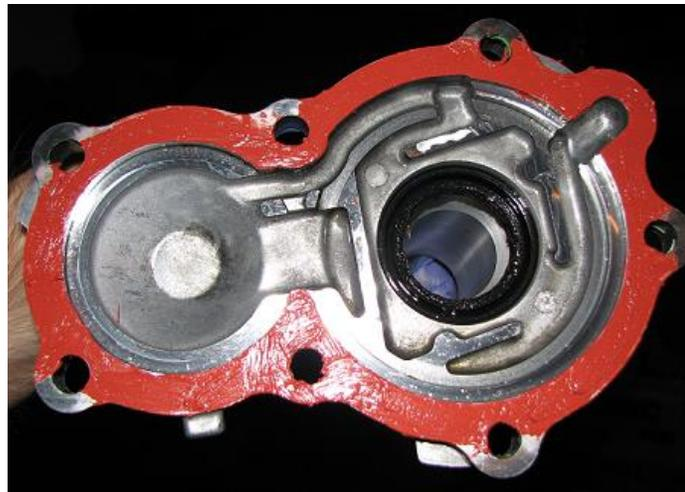
35) Install this cover with the (7) 12mm bolts using thread sealant on the threads. Torque to 13 ft-lbs.
