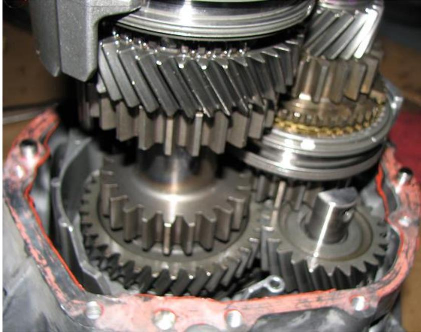
32) Temporarily install one of the 12mm reverse idler bolts with a gasket and install the oil receiver tube insuring it is correctly in all the necessary grooves. Use of a flashlight will be necessary. These are shown below.
