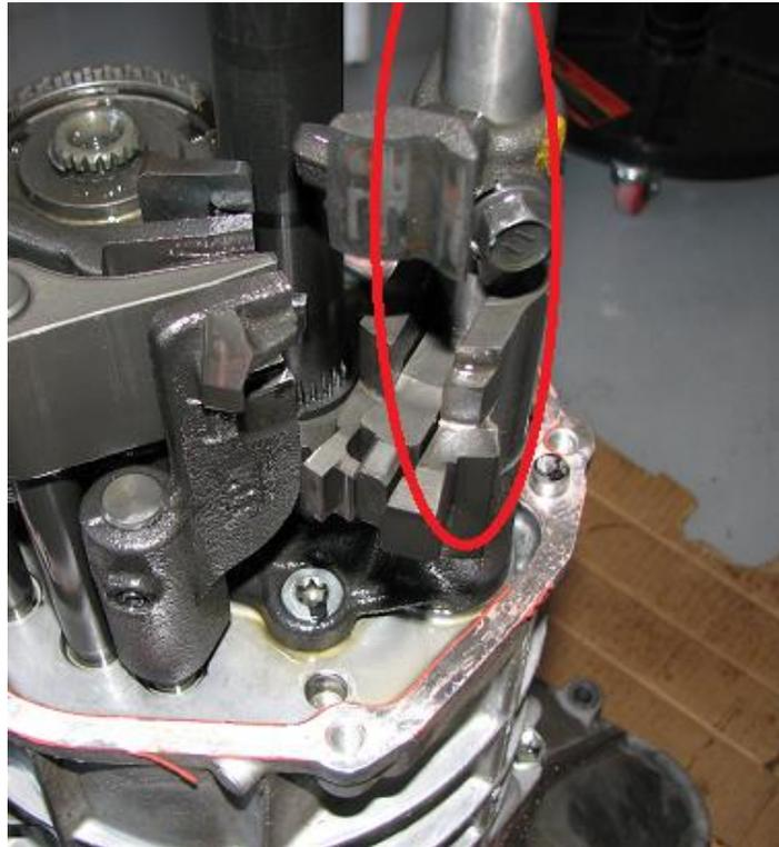
11) Using a T40 torx socket, remove the 3 detent bolts. The green two, you will want to use a magnet to remove the spring and detent ball as well from the hole.
