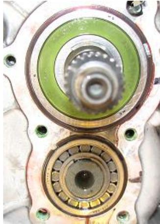
34) Using Toyota's Transmission Sealant (orange), apply sealant to the front cover as shown below. Use grease or generously apply transmission oil on the seal to decrease the chance of ruining the seal.
