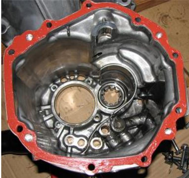
37) Place the transmission case on the bell housing and push it down onto the dowel pins. Using an adhesive (blue Loctite is appropriate) to resist the bolts backing out, tighten the (9) 12mm bolts. Torque spec is 21 ft-lbs. Place the bolt with the wire harness ring on the top side (shown below in red).
