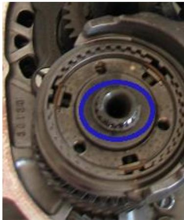
16) Using a steering wheel puller (aka Toyota/Subaru's SST), remove 6<sup>th</sup> gear's synchro hub from the countershaft assembly.
