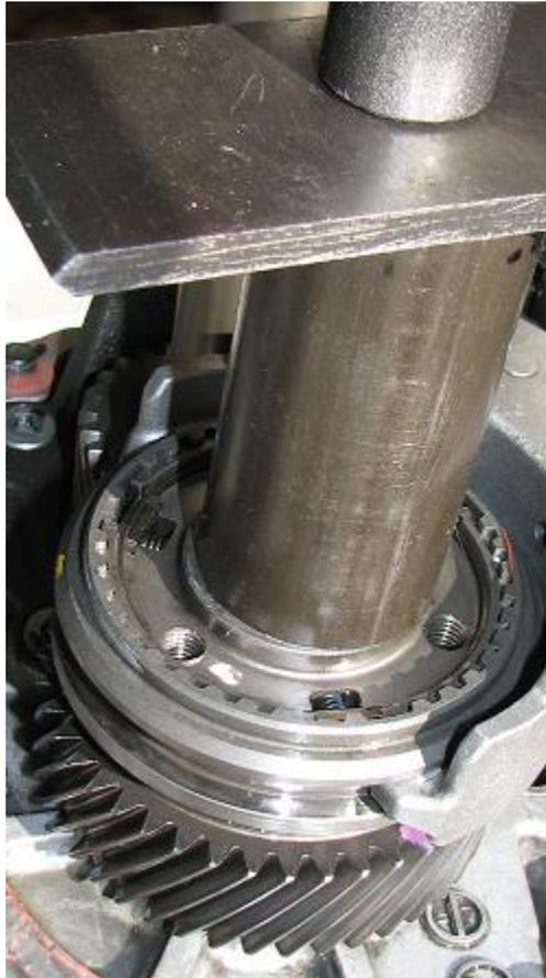
44) Install the snap ring on the top of the counter shaft.
