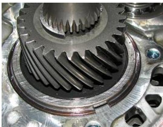
40) Grab the rear bearing retainer and re-install that over the output shaft's bearing. Using Loctite on the T45 torx bolts, tighten the (4) bolts to 22 ft-lbs.
