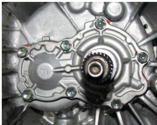
36) Using the same orange Toyota FIPG sealant, spread a nice even sealant ring to the transmission case as shown below.
