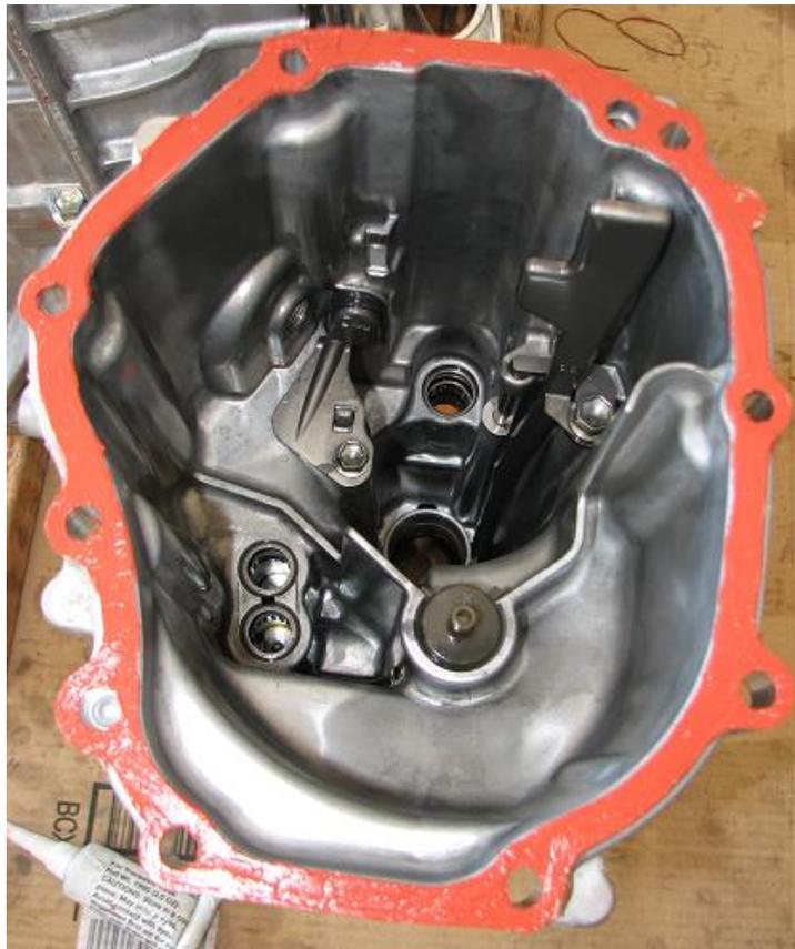
56) Install the tail section and install the (8) 12mm bolts to 21 ft-lbs.
