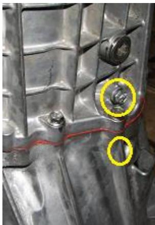
39) Install the output shaft snap ring with a snap ring expander.
