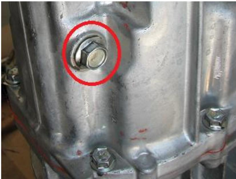
58) Install the 27mm holder with a spring and detent inward in the trans as shown below. Torque to 29 ft-lbs.
