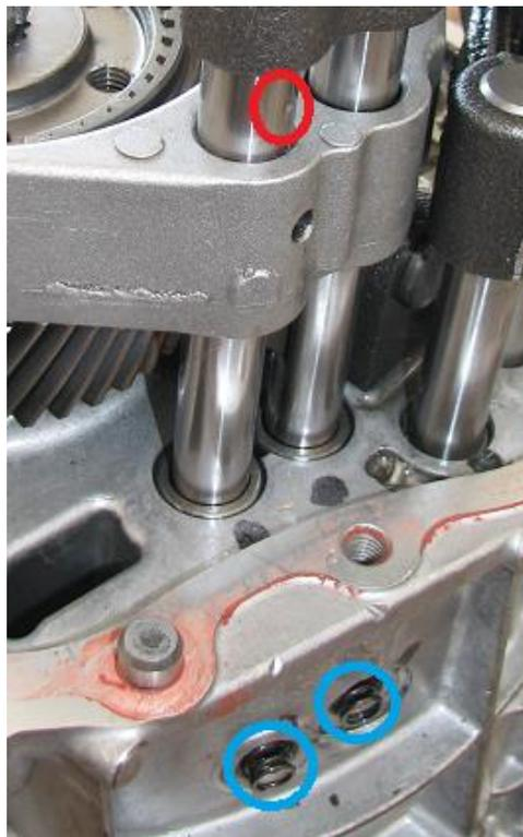
52) Install the T40 torx with a dab of sealant in the (3) transmission case points. Torque to 14 ft-lbs.
