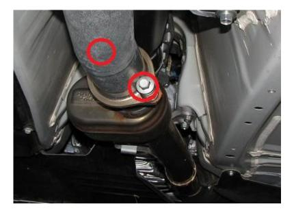
2.4. With the exhaust removed, we start with removing the center part of the driveshaft by removing the two 14mm bolts circled in yellow below. This will cause the driveshaft to droop in the middle.
