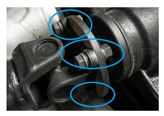
2.6. Using the small pry bay, pry the driveshaft off the rear differential. When this happens, the yoke will want to slide out of the transmission so be careful.
