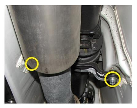
2.5. We now need to remove the 14mm that connect the driveshaft to the rear differential. There are (4) of these, you will want to use a wrench on each side to remove these. You will likely have to use the e-brake to stop the driveshaft from spinning and do this twice to reach all (4) bolts/nuts. Place these bolts/nuts to the side as we will need to reuse them!
