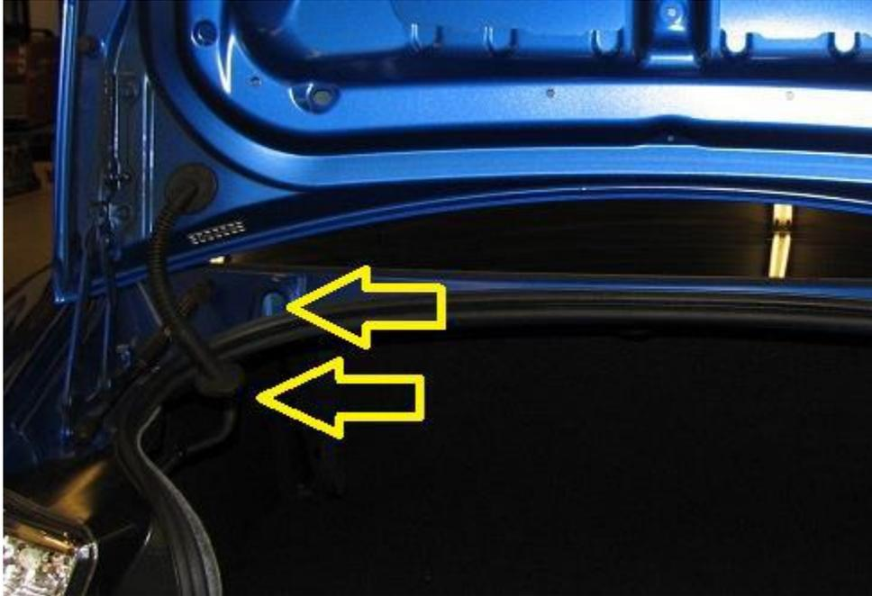
2.4. Remove the trunk shock from the trunk with a small flat head screwdriver, as shown below.
