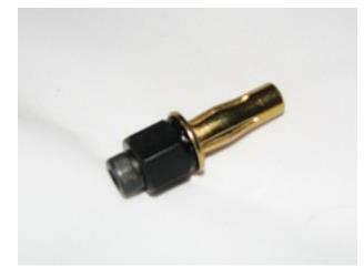
3.6. Place the rivet nut into the hole. If you'd like to use the rivet nut backing washer, you'll need access to the top side of the material you are riveting onto. Note, the backing washer is not necessary but will decrease the chance that the rivet gets pulled through the bumper.
