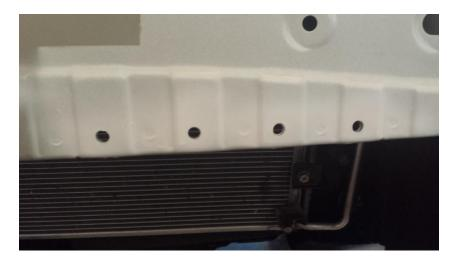
**4.10.** Ensure that the brackets will fit and that they can slide together till there is a 10mm gap between the two mounting holes for the splitter tie rods. Do this by using the (8) M6 x 1.0 x 16mm long BHCS, (8) M6 x 18mm, and the (8) M6 x 1.0 flanged nuts. You do not need to tighten these down, just enough to know if the brackets will work once the bumper is put back on. Once you ensure the holes were drilled properly, remove the brackets and reinstall the bumper in reverse order
