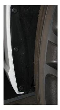
**4.5.** The turn signal has to be removed to expose the final plastic push pin and then the front bumper will come off. There is a metal tab that needs to be push towards the **\*front\*** of the car. The arrow in the picture shows this well. I used a flat head screwdriver to push this forward and then gently pried the signal away from the car.
