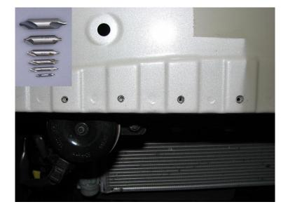
**4.9.** Using the 1/4" drill bit, drill through both parts of the sheet metal. Vacuum out all of the metal shavings you can. It is recommended to spray the holes with spray paint (at the very least) and underbody rust resistant if you have some. This ensures that the crash beam will not rust for years to come.
