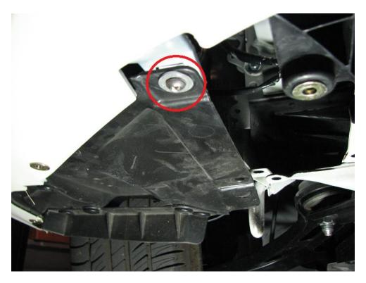
**3.11.** Install the splitter with the M6x1.0 x 30mm BHCS with large washers on each of the rivet-nuts. Utilize the aluminum spacer and the 30mm long BHCS on the two most rearward holes. We suggest to leave all bolts loose until they are all in and then tighten from the inside out. We also suggest you have the splitter held up by 4 or more bolts before letting the splitter free hang.
