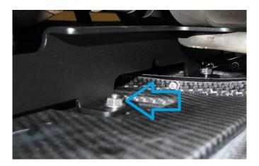
**2.15.** Moving to the rear location, we perform a similar operation. Nuts on top of the bracket, with a bolt and washer on the bottom of the diffuser. It is possible to reach your hand in through the rear to get the nut on the bolt. Alternatively, you can use a cat claw/lady finger to hold the nut in location.
