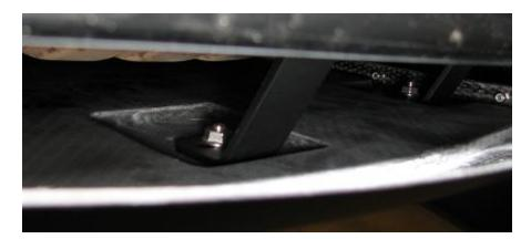
**2.16.** To install the center forward most nut; use the lady fingers again to position the nut in the correct location.
