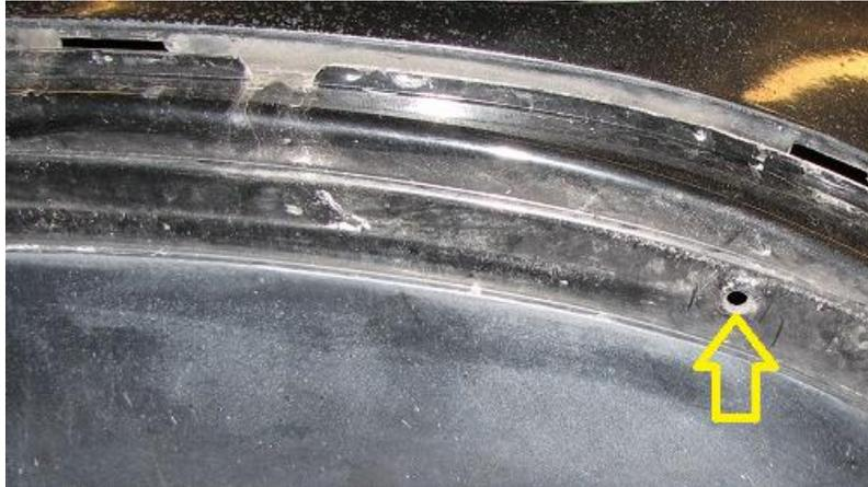
**2.6.** We want to open these holes to 3/8" with a drill and drill bit.
