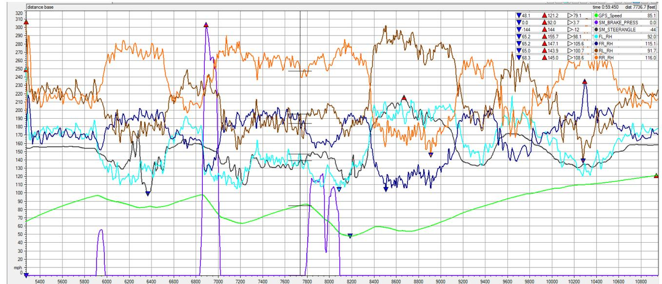
Ride heights correlated with downforce numbers when corrected for weight transfer and roll. We are still working on optimizing suspension setup to go with the added downforce.
