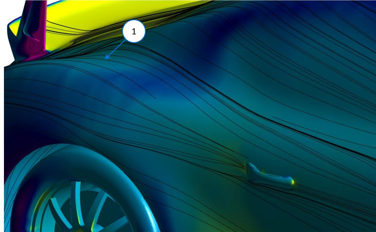
1. The flow structure towards the rear of the car can be seen in both images. The streamlines flow up the rear quarter panel and towards the center of the car. This can be seen in both the flow viz and CFD. The flow field is a little stronger on the flow viz and this indicates the door handle has less interaction to the flow than in CFD. This is very minor but can be noted by careful examination on the flow viz.
