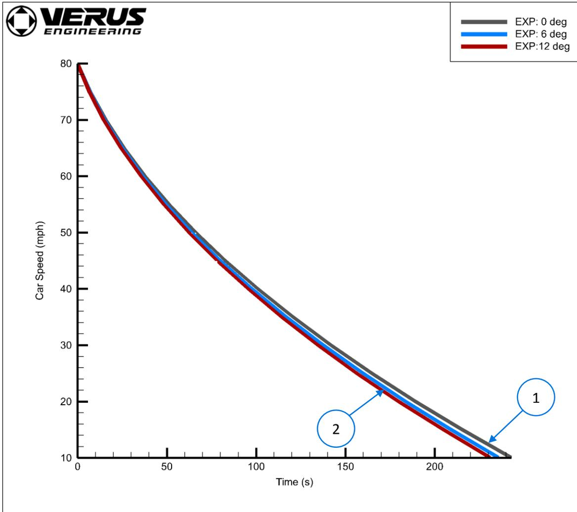
We followed the SAE standard of coast down testing as close as we could. We coasted down from 80mph to around 10mph with 3 different cases; wing at 0 deg, wing at 6 deg, and wing at 12 deg. The data was recorded using an AIM data logger and 4 runs were done and then averaged. Elevation changes were ignored because it could not be accurately calculated. Runs were made on the same day, at the same location, back to back.
