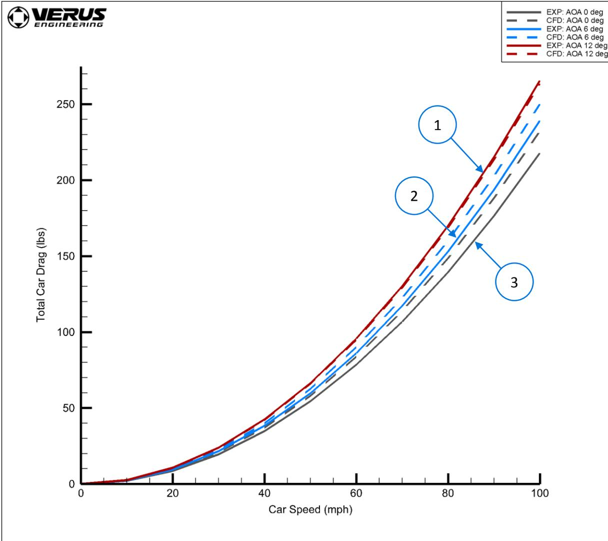
From the coast down testing data, calculation of the coefficient of drag (cd) was completed. From this, the ability to compare simulated CFD drag to coast down testing drag was possible.
