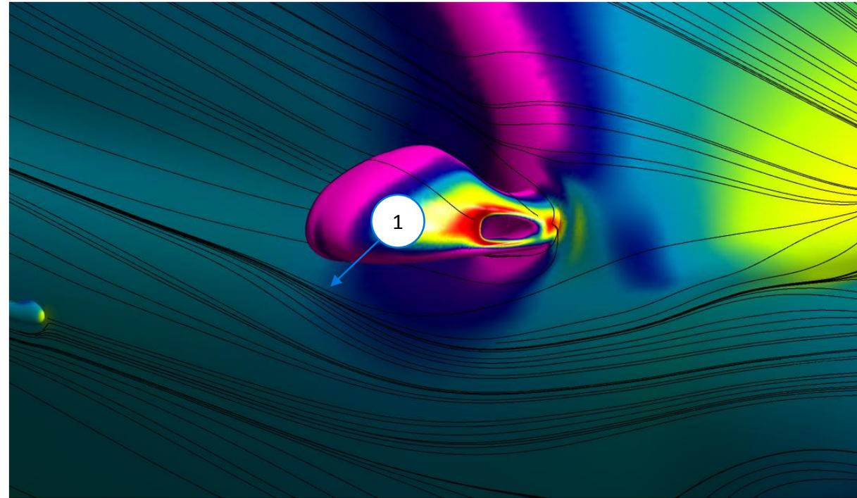
1. The flow structure around the mirror is the same in CFD and flow viz. The streamlines can be seen coming from the top of the fender/hood, down the door, under the side mirror, and then curving up before straightening out. This flow field is caused by the shape of the car and the mirror. The low pressure on the bottom side of the mirror causes the flow field to curve back up while the high pressure on the front side causes the air to flow down in the front of the mirror.
