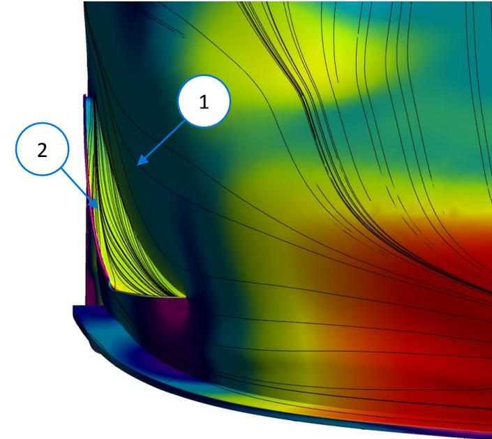
1. The flow field on the bumper can be seen traveling up along the dive plane and rearward. This is also evident in the CFD image and can be seen very easily. This is from the interaction of the high velocity field around the bumper and its interaction with the dive plane.
