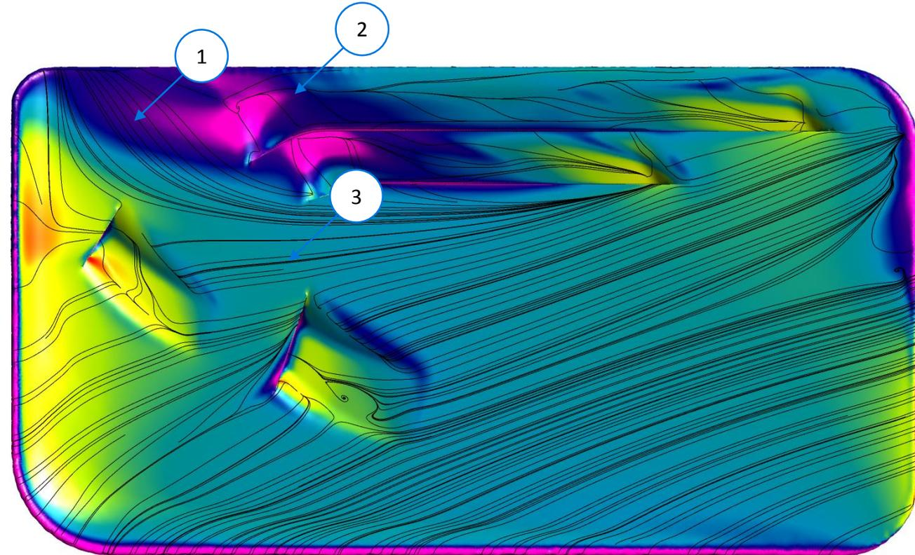
1. The flow viz and CFD flow line up very close on the endplates. The flow can be seen on both curving up and rearward on the endplate.
