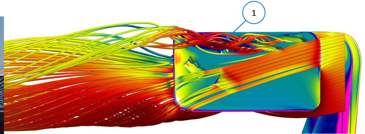
1. The tufts can be seen flowing from the high pressure side (top inside) to the outside. This is also seen in CFD and the vents were specifically designed to operate this way. The geometry is very critical for this to work right and is also dependent on the airfoil shape.
