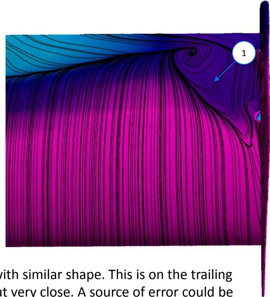
1. Separation can be seen in the flow viz and CFD in the same location with similar shape. This is on the trailing edge of the wing and close to the endplate. The shape is a little off but very close. A source of error could be cross winds during testing.
