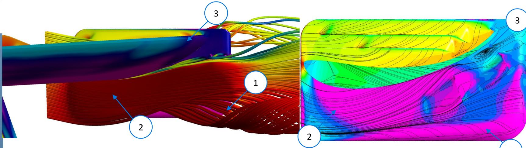
1. The airflow around the rear bottom of the endplate travels down and rear. This is because the air is trying to go under the end plate to the other side which creates a vortex. This design decreases the strength of this vortex.
