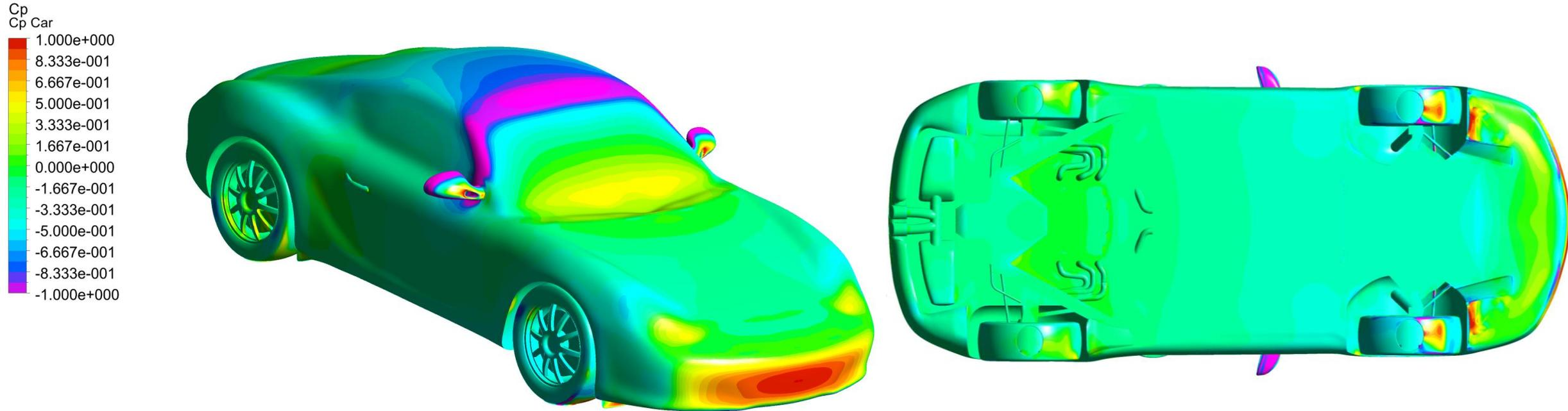
Analyzing the vehicle's baseline is the first step in the development. This gives our team the starting point and locations where improvement can be developed. From there, we can make incremental changes while watching how these changes impact drag, downforce, and aerodynamic balance.
