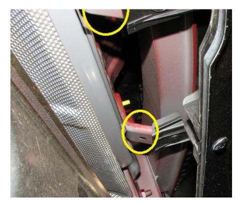
**2.13.** Grab the long, rear mounting brackets. These install with larger angle attaching to the chassis and the sharper angle will bolt to the diffuser. Use an M6x1.0 x 20mm long bolt and
