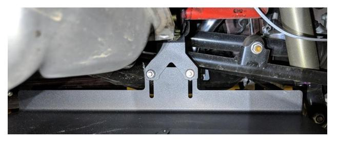
**2.18.** Moving rearward, install the rear two locations. Install height will determine if you use the 20mm long M6x1.0 bolt or the 35mm long bolt. If the diffuser is installed low, longer bolts will be required with more spacers. If the diffuser is installed relatively high up, the shorter bolts can be used. Shown below we used the 5mm spacers.
