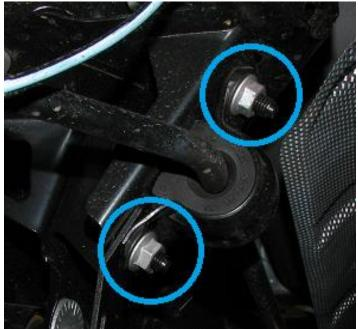
**2.27.** Tighten the outside (4) mounting points with the 4mm allen wrench. The serrated nut should not need held as it will resist turning while you tighten the bolts.
