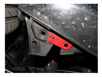
**2.12.** Moving rearward, we find the two rear most mounting points for the diffuser. These locations are circled in yellow below.
