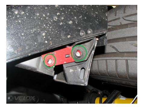
**2.10.** Reach up into the fender liner and remove the (2) plastic clips on each side of the rear bumper. These clips are shown below, removed.
