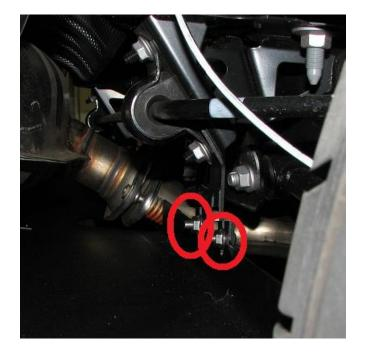
**2.26.** Tighten the front bracket to sway bar points which are 12mm hex head bolts to 16 ft-lbs (circled in blue).
