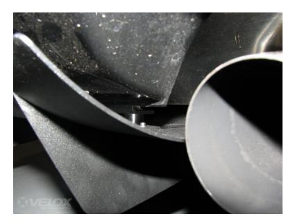
**2.19.** Once again the button heads are on the bottom with a washer, and the nut goes on top.
