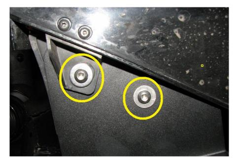
**2.28.** Finally, tighten the rear two M6 x 1.0 button heads with the proper spacer used.
