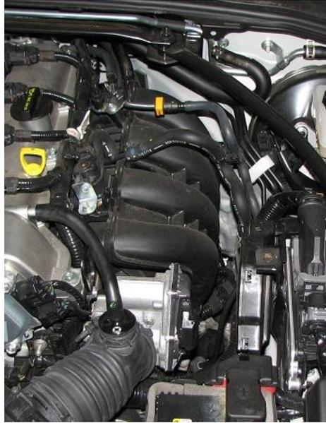
**2.6. With the Verus Engineering AOS, we filter the airflow from both the PCV vent as well as the valve cover vent.** We will leave the easy hose connections (valve cover to intake, orange arrow) till the end and work on the hardest part first; the intake manifold to block PCV valve connection (blue arrow). This is located under the intake manifold and towards the firewall of the engine bay.
