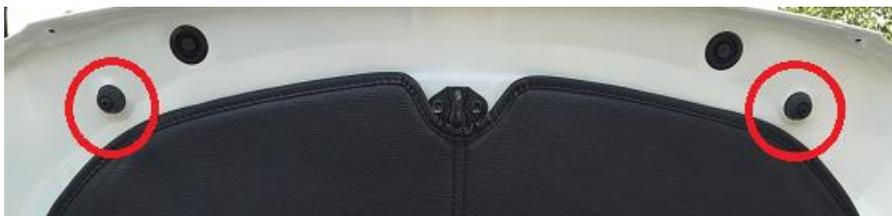
**2.14.** Open up the holes to 3/8" using the step drill bit.
