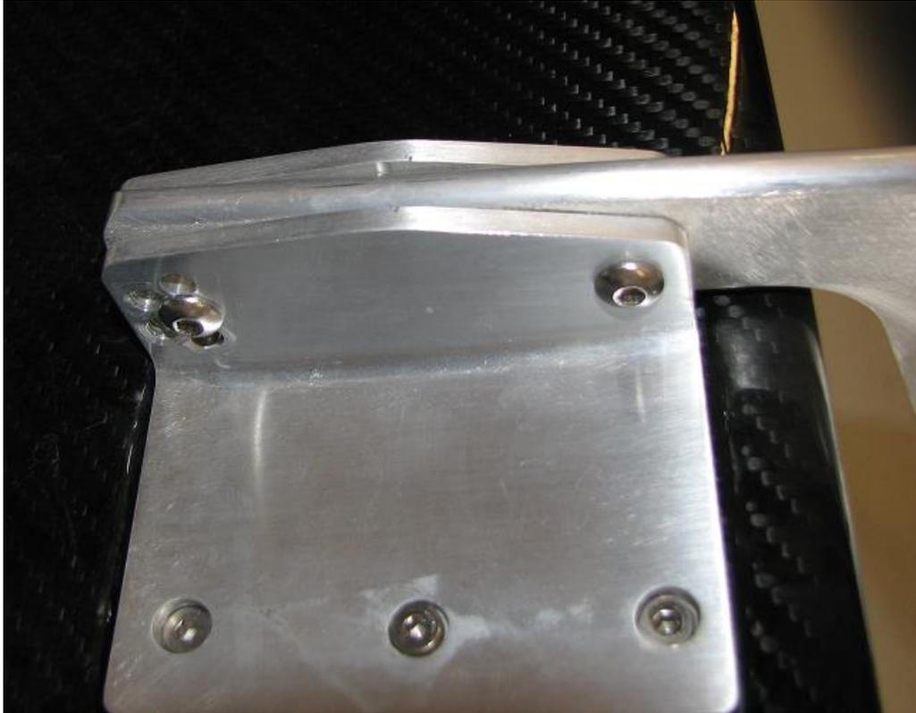
**2.12.** The rear wing is now installed on the trunk and we only have one more part of the install, which is the trunk load transferring rivet nuts and bolts.
