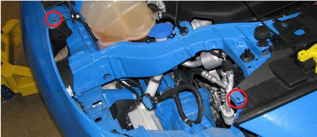
2.9. With the front of the car off the ground, we will want to start by removing the underbody plastic vertical piece. You remove this by unscrewing the (3) bolts circled in red below. This will be removed and left off.
