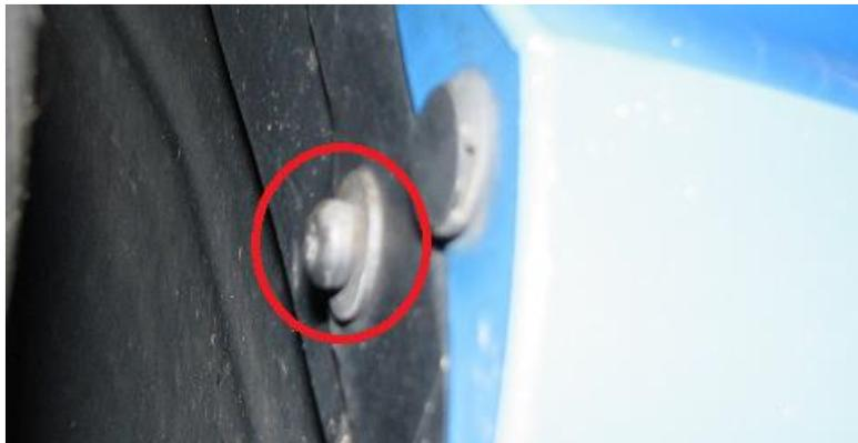
**2.32.** Locate the other (4) locations that we will install the clip-on nuts. Two of these locations are shown below.
