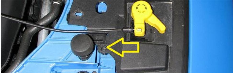
2.8. Remove the headlights from the vehicle by removing the two bolts holding it in. These are circled in red below, but the headlight is already removed.
