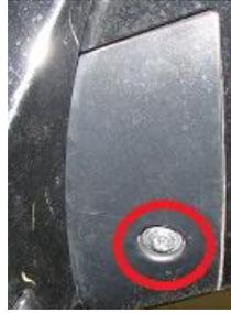
**2.4.** Remove the two Torx bolts shown below on each side of the wing.
