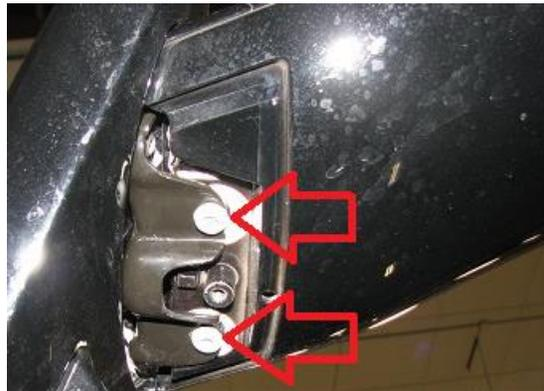
**2.5.** To remove the wing, pull outward on the factory upright and pull up and out on the rear wing. Below is a photo with the factory wing removed.
