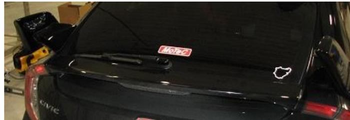
**2.6.** With the OE wing removed, we can install our upgraded wing in place. Do so in reverse order by placing one side on the mount and pulling outward on the other upright.
