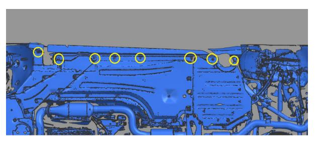
2.4. Grab one of the side splitters and note the diagram below for bolt, washer, and spacer locations. The black logo plate is intended to be facing upward and at the rear of the vehicle but can be installed downward if you prefer that look. Keep in mind, the spacers need to be placed between the side splitter and the factory side skirt mounting location. (THCS > washer > side splitter > spacer(s) > factory side skirt mounting hole)
