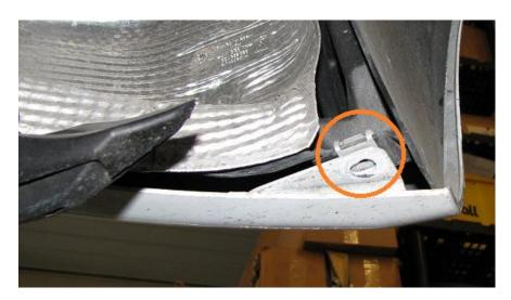
**2.12.** We can now work on installing the diffuser panel. To do this, pull down on the fabric panel and come in from the side. The panel will go above the NACA duct circled in yellow below. This gives you an idea of how low to pull down on the fabric panel. Doing this will allow the panel to get into place.
