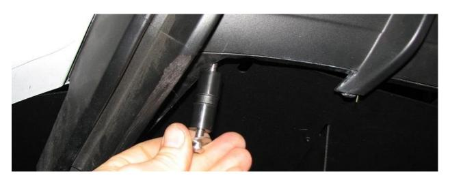
**2.17.** We will reuse the outside most bolt as well, which is the T30 coarse thread bolt with a shoulder, as shown below.
