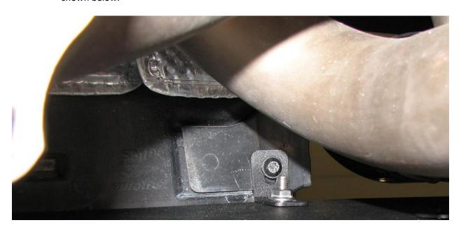
**2.10.** Next, we remove the T25 bolt and factory clip on nut. We replace this with the supplied M6 clip on nut which is shown with the green arrow below. This is the green circle in step 2.4 above as well.
