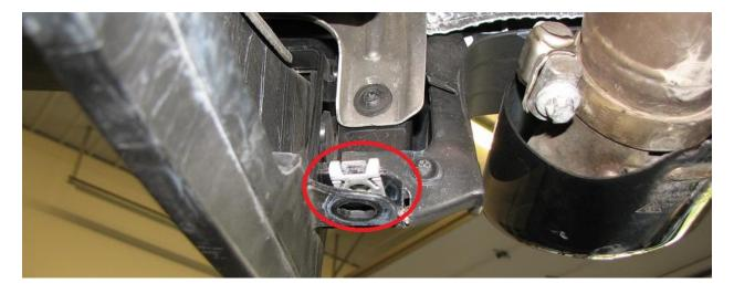
**2.8.** Remove the T25 bolt shown below, circled in blue in both step 2.4 and below.
