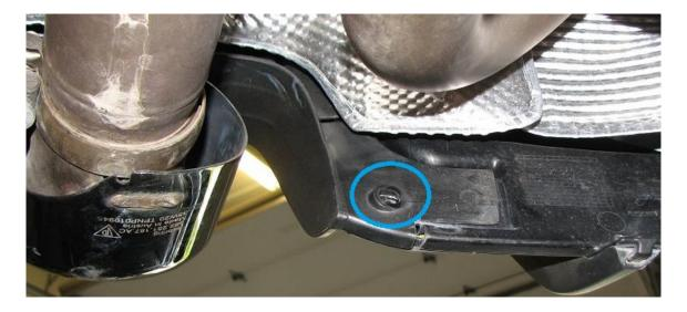
**2.9.** We will install the bracket in this location by reusing the factory bolt. Install the bracket as shown below.
