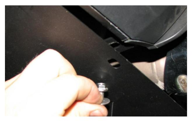
**2.16.** The next location moving outward will be using the 60mm long BHCS, washer, (2) 15mm long spacers, and (1) 5mm spacer. The bolt and washer go on the bottom side of the diffuser, and the spacers go above the diffuser. To install the spacers on top of the diffuser,
