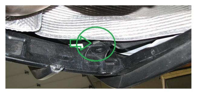
**2.11.** Finally, remove the T30 bolt circled in orange in step 2.4 and the below image.
