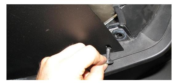
**2.15.** The next location outward, which bolts to the bracket we installed in step 2.9, we will use the 16mm long BHCS, washer, and the serrated nut on top. This is shown below.
