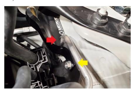
**2.7.1.** Temporarily unbolt the Brake Master Cylinder Brace, and install the supplied foam tape to the A/C line so that it prevents contact with the Brake Master Cylinder Brace. Reinstall the Brake Master Cylinder Brace as in **2.7**.
