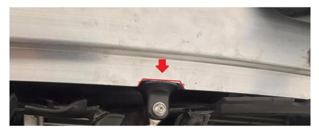
**2.7.** On the bottom side of the crash bar, hold a clevis up, center it, and make a mark. Follow up with a center punch to aid in drilling.
