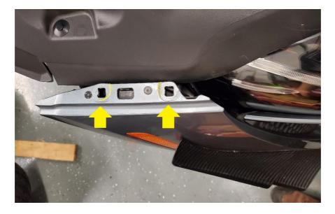
**2.4.6.** Disconnect the connectors on each side of the bumper, and unclip them from the chassis.
