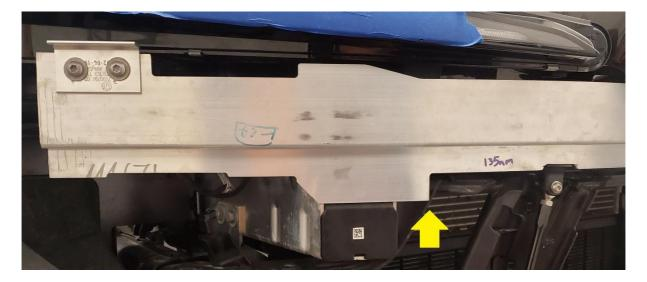
**2.6.** Mark about 13mm or 1/2" on either side of that mark, and remove the lip so that the clevis can sit flat on the bottom surface of the crash bar.
