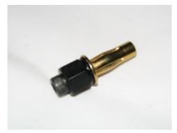
**2.10.** Using the 9/16" wrench and the 5mm allen wrench, hold the rivet nut install tool steady and tighten the allen bolt. You will have some initial resistance, then the rivet nut will begin to pull tighter on the material.
