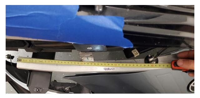
**2.13.** Assemble the support rod as shown. Note: There is a left-hand thread and a right-hand thread rod end.
